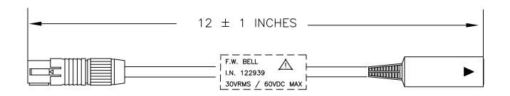
The 122939 adapter cable is designed to connect standard GaAs 5000 Series probes to a 5100 Series Gaussmeter. It has no active components and is an interconnect device only.
