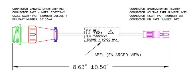
THE ADAPTER (ITEM NUMBER 122938) IS USED TO CONNECT A 9200 GAUSSMETER PROBE TO A 6000 SERIES GAUSSMETER. IT HAS NO ACTIVE COMPONENTS AND IS DESIGNED AS AN INTERCONNECTION DEVICE ONLY.
