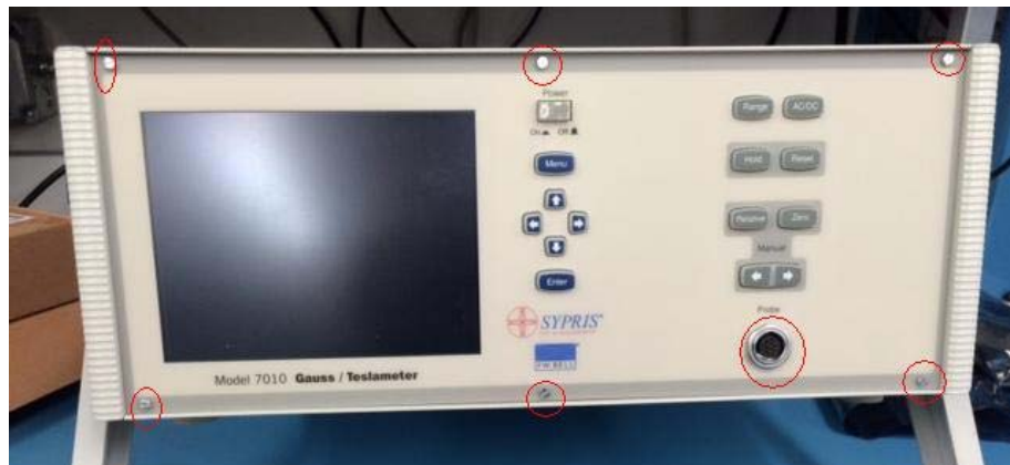
Figure 1 Remove screws and probe connector nut
