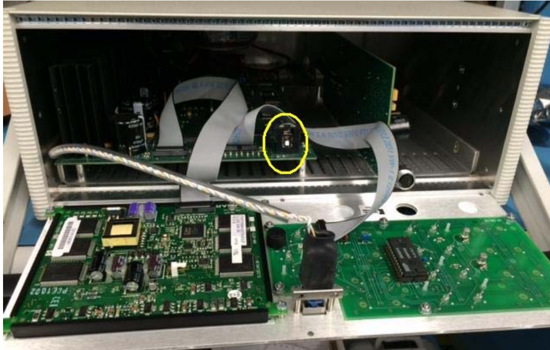
Figure 2 Front panel tilted down to access battery (yellow circle)
