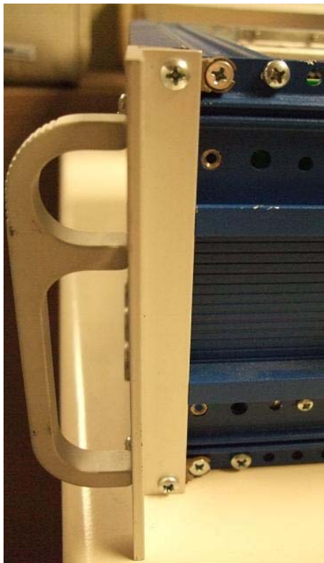
Photo 6 - Side screws w/star washer in bracket
