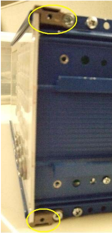
Photo 4 - Spacers Installed on case
