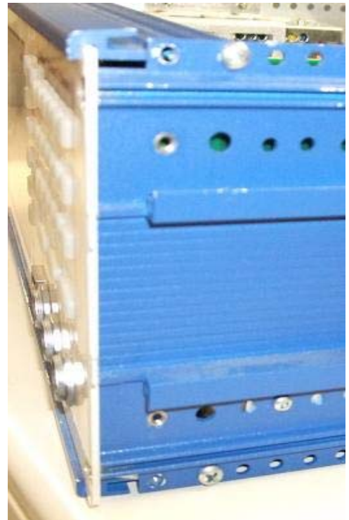
Photo 3 - Corner piece removed
