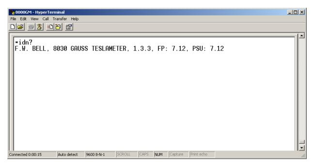
After connection to the meter is established, any of the SCPI commands described in the meter's instruction manual can be used to provide remote access to both settings and measurements.
